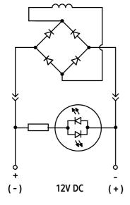
version with cable box and light signaling LED -...|WE6...1X/...DL
